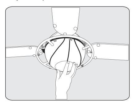
Screw in Compact Florescent light bulb (included). Place Light Kit Lens over bulb screw into place.
