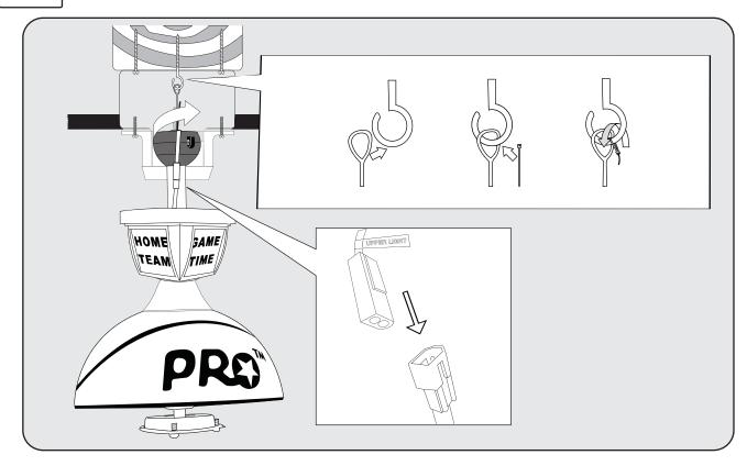
Lift fan onto the mounting bracket (1). Turn housing until hanging ball seats itself into ball socket (listen for click).
