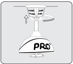
Seat the canopy screw cover into slots and twist to lock.
