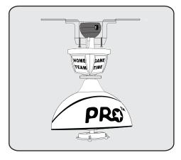
Attach Canopy Night Light (3) to the mounting bracket by placing canopy screws into keyed hole slots.
