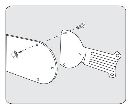
Assemble Blade (11) to Blade Arms (8) by inserting screw (S4) and securing with Blade Medallion (10).
