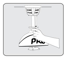
Tighten screws firmly.
