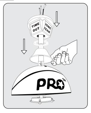
Place flange cover (4) over downrod assembly. Place canopy screw cover over downrod. Place Canopy Night Light (3) over downrod (2).
