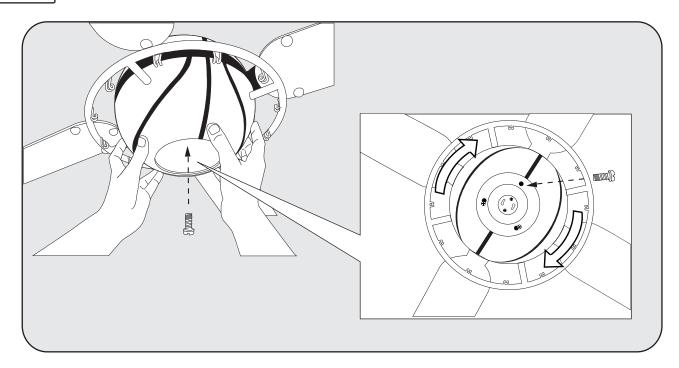
Seat Light Kit (5) into position and lock into place by twisting 1/4 turn. From light kit hole screw set screw into place firmly.
