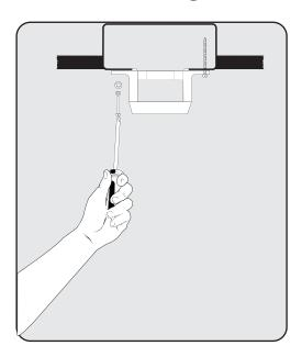
Prior to securing mounting bracket, screw "J" hook (S7) into ceiling outlet box as a secondary support means. Secure mounting bracket (1) to the outlet box (A) by tightening bracket screws & washers (S3) as shown. If not mounting to an outlet box, use wood screws (S1) and washers (S3) and mount securely to ceiling beam.
