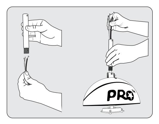
Insert fan wires through downrod.
