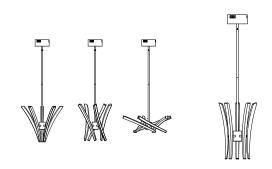
*Note*: The arms on the LED fixture can be moved to the desired position.
